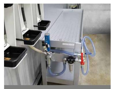
Custom 2m long waste oil tray with attached Pneumatic pump, filter, and hosing
