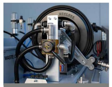
Waste Oil 4-Way Evac Valve and Suction Hose Reel incorporated on to a mobile service skid
