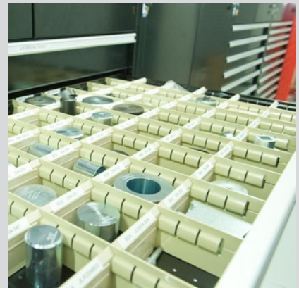
Traditional high density BAC Drawer customised for special tool storage
